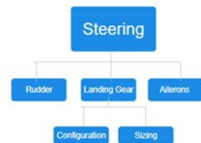
Figure 9: Steering Functional Decomposition
